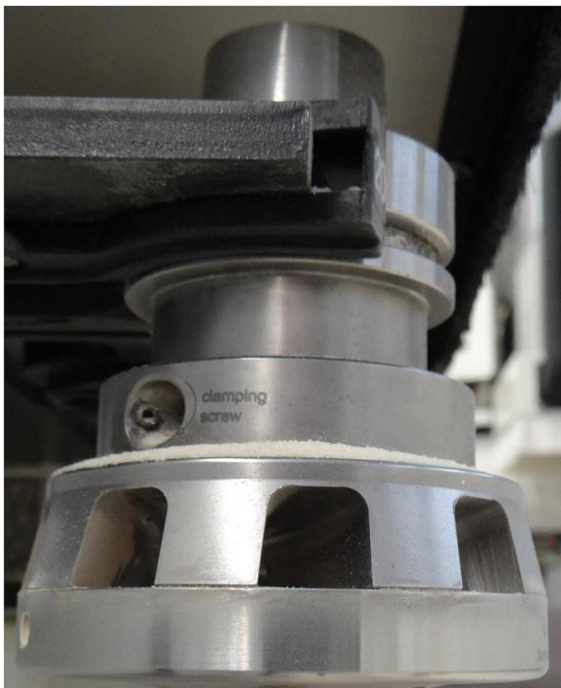
The second screw is used to un/clamp the tool, which can be done with an ordinary screwdriver, most often an Allen key. Hydraulic chucks are often also manufactured with a dust extraction turbine for nesting formatting technologies.
