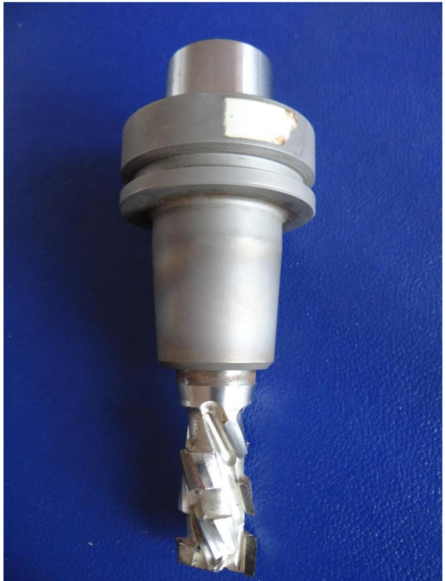
extremely tight clamping of the tool. In addition, this clamping is extremely precise and is therefore suitable for high-performance tools. The disadvantage thus remains only the high price of the clamping device and the consequent need to change the tool in the form of a service which is not expensive, but it is necessary to wait for the tool change service. The disadvantage is also the impossibility of clamping tools with a large diameter, since the heating ring is limited by this parameter.
