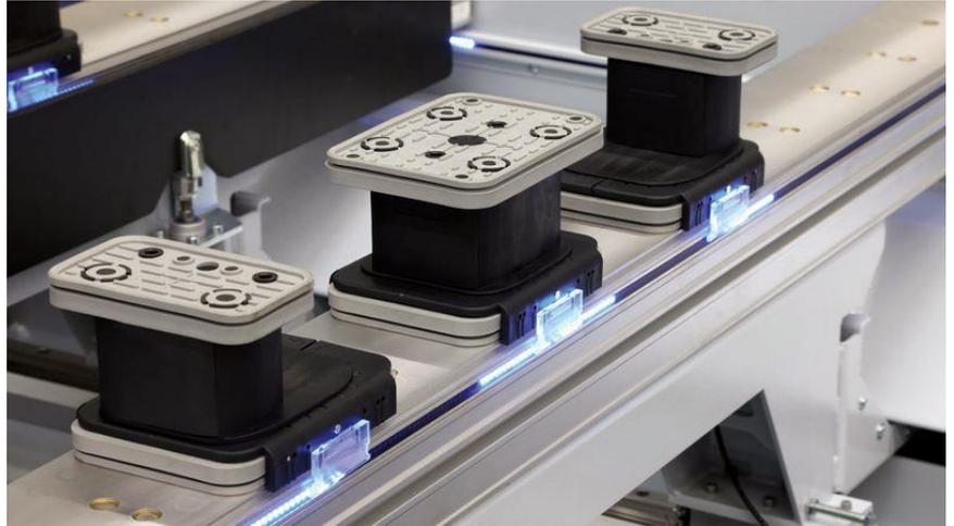
position of the suction cup, which was designed in the CAM section of the table equipment. Some manufacturers use a single-color system, others use a traffic light system (red, orange, green). The big advantage is the possibility of operation without moving the machine portal/boom, unlike the cross laser, at the same time this solution is significantly faster.
